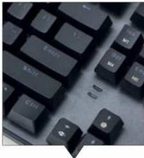
The double-shot molding process ensures that the legends will never fade.
