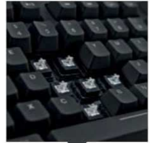
The Celeritas II uses Adomax Flaretech optical switches.
