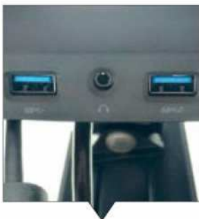
A pair of USB 3.0 ports flank a headphone jack along the bottom bezel, ideal for a keyboard and mouse combo or for connecting flash drives.
