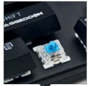
The Outemu Blue switches here are modular and hot-swappable.
