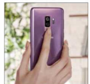
The main rear camera on both phones is a dual-aperture lens that switches between f/1.5 and f/2.4
