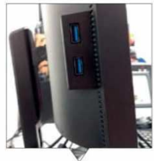
There are a grand total of five USB 3.0 ports, two of which sit off to the monitor's side for easy access.
