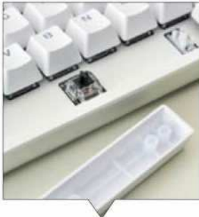
The spacebar is the only key to use a heavier TTC Black switch.
