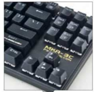
The keyboard uses fairly thick pad-printed legends.
