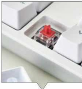
The rest of the keyboard uses TTC Red switches.
