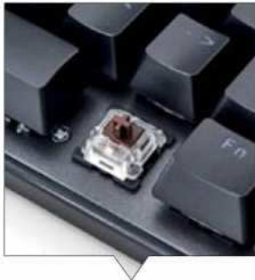
The switches can be replaced with a different switch type.
