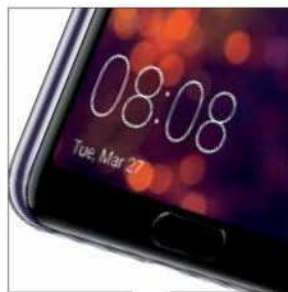
The fingerprint scanner doubles up as a navigation bar.
